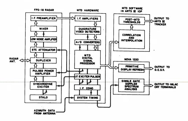
FIGURE 6 MTD System Functional Schematic
