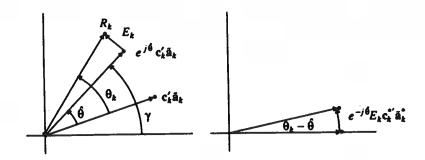
In the right figure above, the entire orientation is rotated by  $-\stackrel{\bullet}{k}$  such that the echo replica,  $e^{j\,\hat{e}}\,c_k\,'\tilde{a}_k$ , appears on the real-axis. This way, it becomes easy to determine whether the phase error  $\theta_k$   $-\stackrel{\bullet}{\theta}$  is positive or negative. If this imaginary part is positive, then the error is reduced by making the estimated phase  $\hat{\theta}$  larger.
