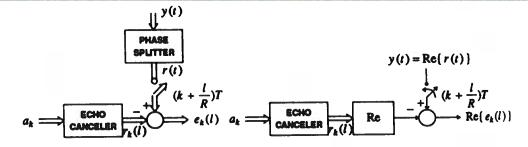
The figure on the left is the one considered so far. It is assumed that the receive analytic signal is generated using a phase splitter, and the echo canceler generates a replica of the echo analytic signal.
