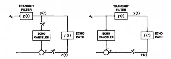
In the left figure, the transmitted data waveform y(t) is sampled at the canceler input, while in right figure, the transmitted data symbols are applied directly to the canceler input so that the transmit filter is included in the echo path.
