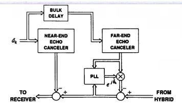
transversal filter, and a phase rotator by angle  $\hat{\theta}_k$  which hopefully matches the carrier phase rotation  $\theta_k$  of the echo channel. The appropriate angle for rotation is determined by a phase-locked loop, which uses the transversal filter output and cancellation error to correct the currently used phase in order to minimize the error signal  $E_k$ .
